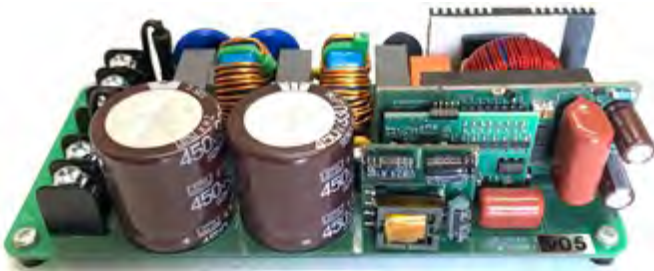
Figure 4: 2.4kW PFC reference design using a totem-pole bridgeless topology and 150V MOSFET switches
