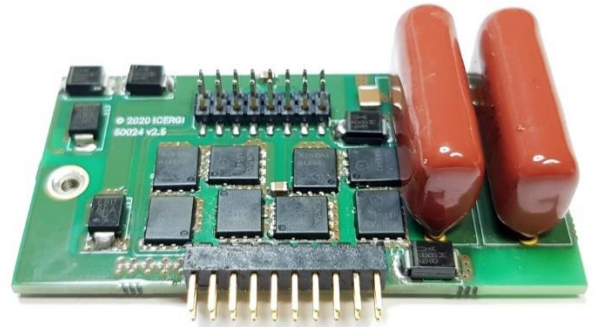
Fig. 9: Power board prototype used in a 2 kW PFC
