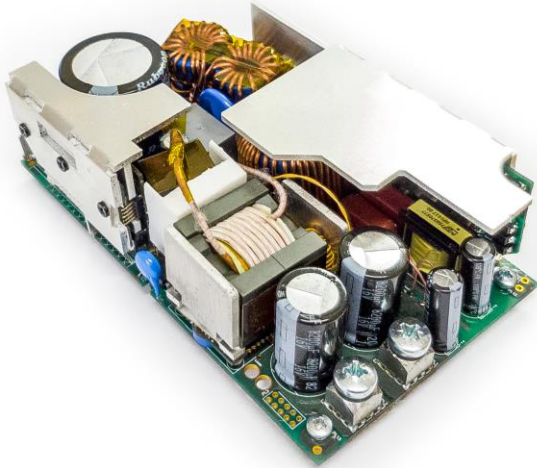
Fig. 2 700W industrial/medical solution in 3”x5” with half-bridge totem-pole topology using ICERGi® drivers and control (left); 700W PFC stage efficiency (right);
