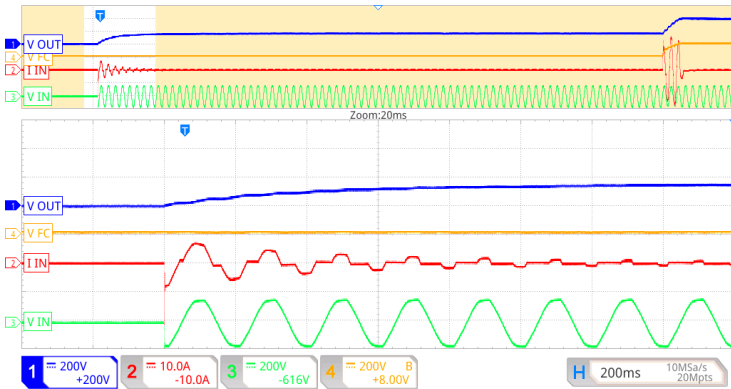
Figure 19: Inrush current waveforms at input voltage V_{IN} = 115V_{AC} , switch on phase angle \Phi = 45^\circ and 0% load
