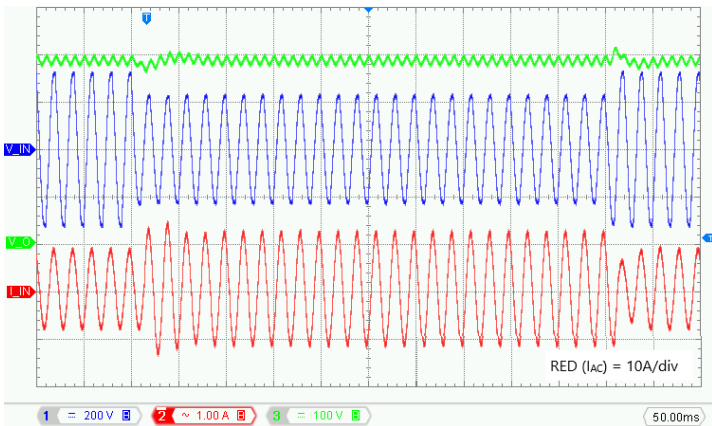
Figure 44: 30% (V AC = 162) input voltage dip (V IN = 230V AC , P OUT = 1300W, V OUT = 400V DC , φ = 0°)
